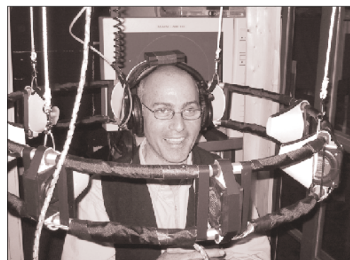
A system for navigation through virtual spaces. Air blows towards the person using the system from the direction of the other person in the space. The sound of the other person's heartbeat is also directional. Project by Bill Meyer.
