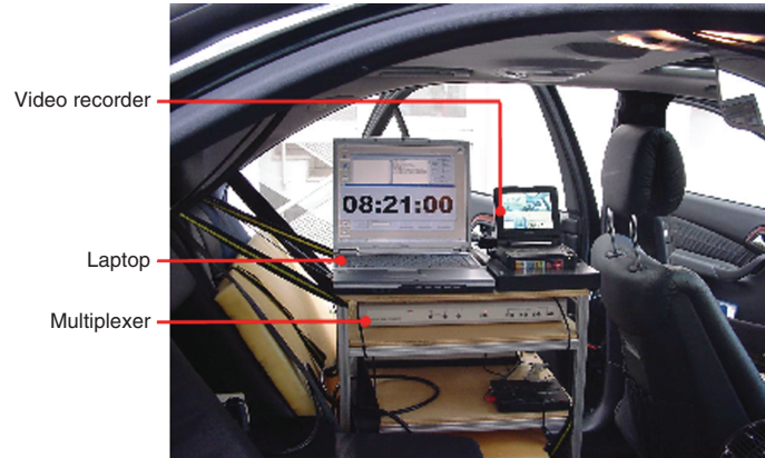
Figure 5. SENECA test car equipment (Mutschler and Baum, 2001).
